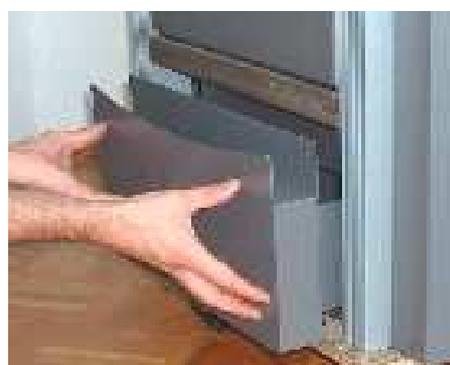
Fig. 15: Replacing the ash pan
