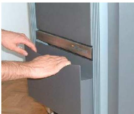
Fig. 14: Removal of the ash pan
